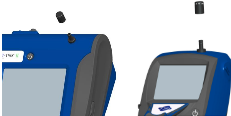
Figure 2-6: Putting on Inlet Cap
