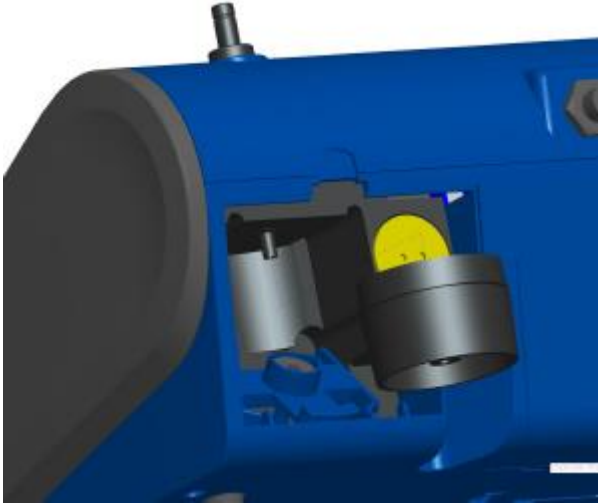
Figure 4-8: Remove 37-mm Filter Cassette
