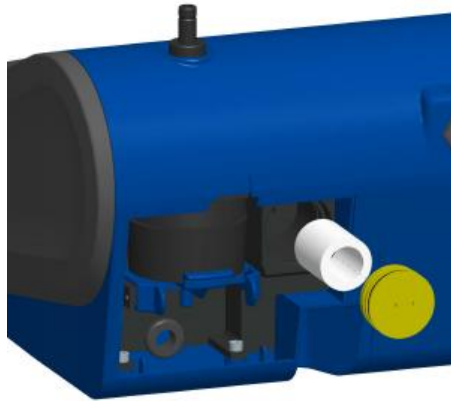
Figure 4-6: Pull out Single Cylindrical Filter from Filter Well (Desktop Model)
