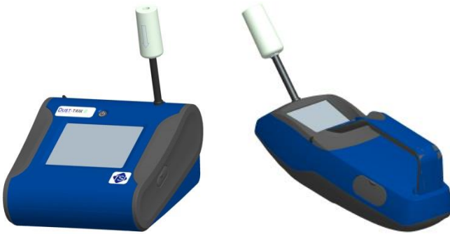
Figure 4-1: Attach Zero Filter to Inlet
