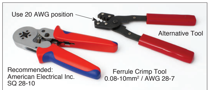
Ferrule Crimp Tool Options (20 AWG)
