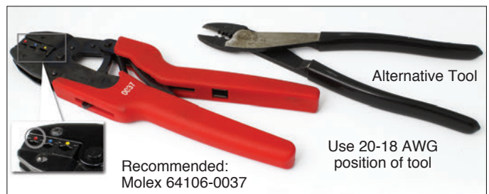
Molex Crimp Tool Options (20-18 AWG)
