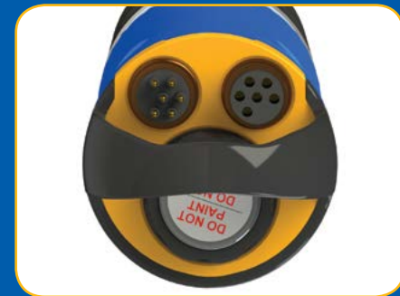
Cable connector, battery valve, and expansion port on EXO2
